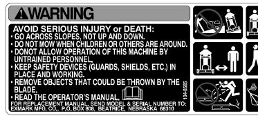
For Units without a Blade Brake Clutch PART NO.: 104-8585 LOCATION: Top LH Surface of Mower Deck
